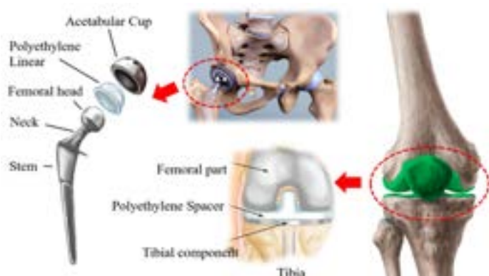
FIGURE 5. Ultra-high molecular weight polyethylene's (UHMWPE) low-friction articulation. 17 (CC by 4.0)
